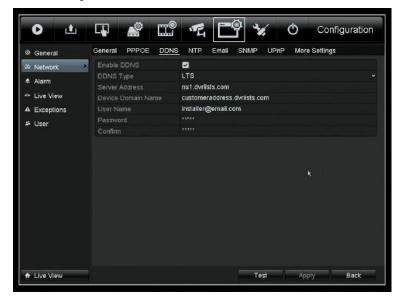
Figure 9. 15 Configure DDNS in DVR/NVR
