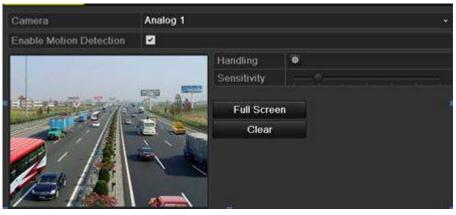
Figure 8. 1 Motion Detection Setup Interface
